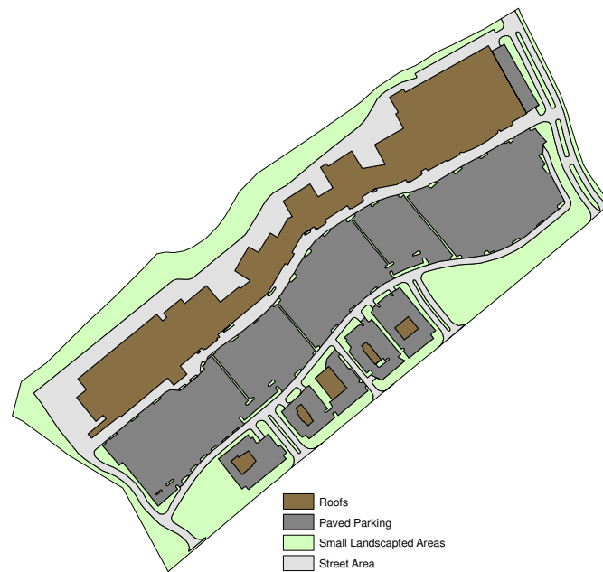
Figure 2-7 Site 1: Commercial Development with Delineated Source Areas
